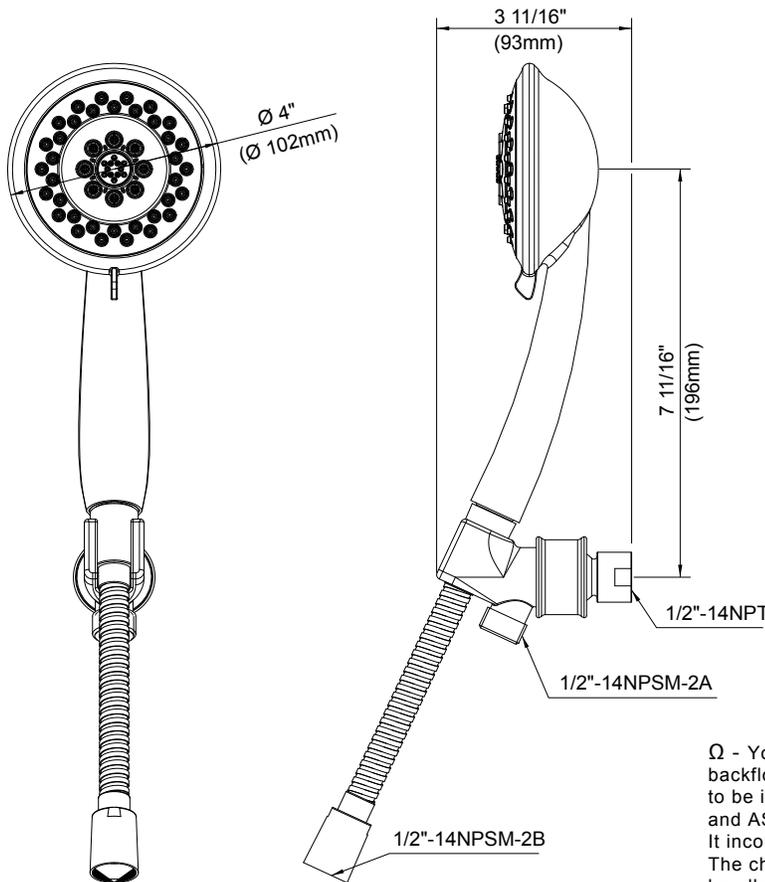
Ω - Your Danze handshower kit incorporates a backflow protection system that has been tested to be in compliance with ASME A112.18.3 and ASSME A112.18.1/CSA B125.1. It incorporates two certified check valves in series. The check valves are located in the handshower handle, and either the supply mount or the showerarm mount outlet.
