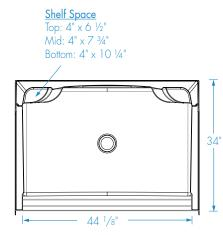
FEATURES Dimensional Tolerance ± 36". Dimensions needed for site preparation should be measured from the unit. Manufacturer assumes no responsibility for preparatory work.
