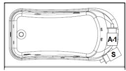
Standard (S) & Alternate (A-1) Pump Locations Pump must be located at A-1 position when ordered w/ a heater
