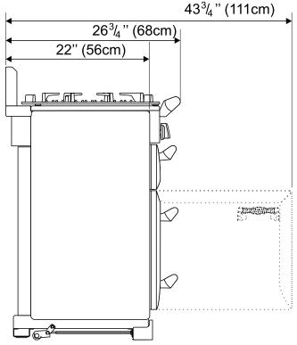
If the range is to be installed between 24" deep cabinets the optional rear spacer should be fitted to move the range 2" forward. See the spacer fitting instruction section of these instructions.
