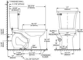
THIS COMBINATION IS DESIGNED TO ROUGH-IN AT A MINIMUM DIMENSION OF 305MM (12") FROM FINISHED WALL TO C/L OF OUTLET. \* DIMENSIONS SHOWN FOR LOCATION OF SUPPLY ARE SUGGESTED. SUPPLY NOT INCLUDED WITH FIXTURE AND MUST BE ORDERED SEPARATELY.
