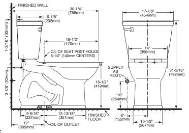
NOTES: THIS TOILET IS DESIGNED TO ROUGH-IN AT A MINIMUM DIMENSION OF 305MM (12") FROM FINISHED WALL TO C/L OF OUTLET. SUPPLY NOT INCLUDED WITH FIXTURE AND MUST BE ORDERED
