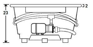
Standard (S) Pump Location and Alternate (A-1) Pump locations.
