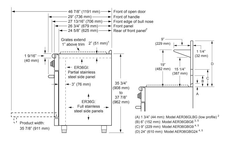
1) Trim thickness is 1/4" (6 mm) with optional self-rimming kit installed (ER36GI only).
