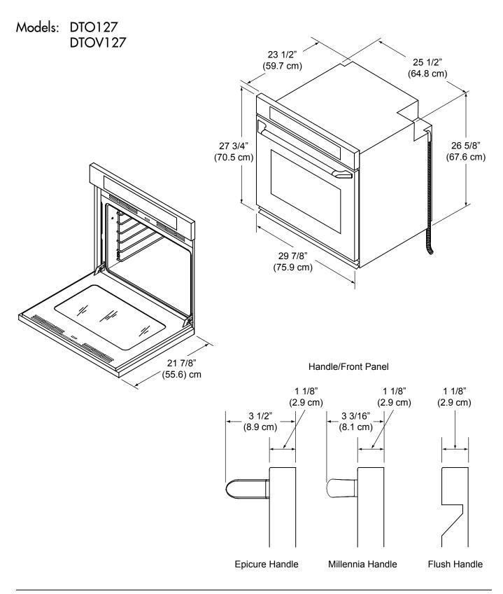
Important: Dacor reserves the right to change specifications without notice. Dimensions provided are for reference only. Before installation, consult the installation instructions accompanying each product prior to selecting cabinetry, making cutouts or starting installation.
