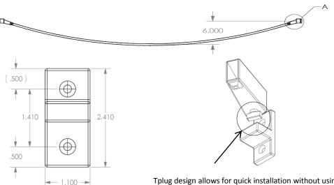
Tplug design allows for quick installation without using set screws to mount shower bar holder to wall bracket
