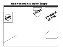
**Reverse plumbing** may be needed in situations where a toilet or sink blocks entry into the tub. In this example, the situation would normally call for a left hand door swing since the plumbing and water supply are on the left. However, since the toilet would block access to the door, a right hand tub would be ordered and the plumber would run the drain and water supply under the tub to the other end. The door and fixtures would end up on the right end of the tub.
