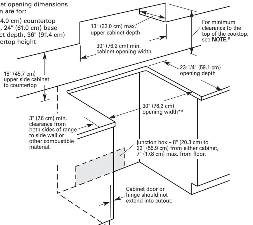
**\*NOTE:** 24" (61 cm) min. when bottom of wood or metal cabinet is protected by not less than 1/4" (6.4 mm) flame retardant millboard covered with not less than No. 28 MSG sheet steel, 0.015" (0.4 mm) stainless steel, 0.024" (0.6 mm) aluminum or 0.020" (0.5 mm) copper. 30" (76.2 cm) min. clearance between the top of the cooking platform and the bottom of an unprotected wood or metal cabinet.
