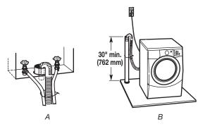
Laundry tub drain system (view C) The laundry tub needs a minimum 20 gal. (76 L) capacity. The top of the laundry tub must be at least 30" (762 mm) above the floor.
