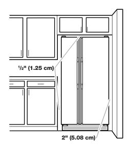
To ensure proper ventilation for your refrigerator, allow for  $\frac{1}{2}$ " (1.25 cm) of space on each side and at the top. Allow for 1" (2.54 cm) of space behind the refrigerator. If your refrigerator has an ice maker, allow extra space at the back for the water line connections. When installing your refrigerator next to a fixed wall, leave a 2" (5.08 cm) minimum space on each side (depending on your model) to allow the doors to swing open.
