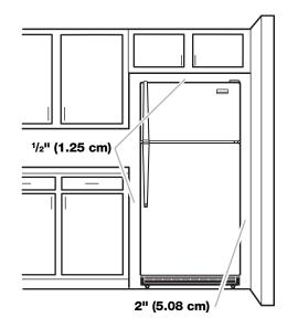
To ensure proper ventilation for your refrigerator, allow for a  $\frac{1}{2}$ " (1.25 cm) space on each side. Allow  $\frac{1}{2}$ " (1.25 cm) of space between overhead cabinets and refrigerator top. Allow at least 1" (25.40 mm) between back of cabinet and the wall. If your refrigerator has an ice maker, make sure you leave some extra space at the back for the water line connections.
