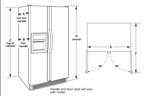
Dimensions "C" and "D" include rollers extended 3/4" (1.9 cm).
