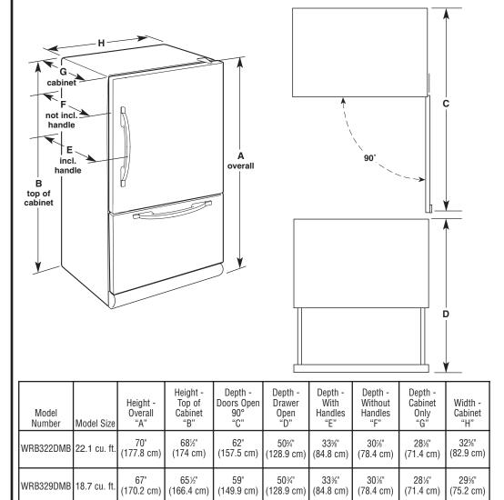
To ensure proper ventilation for your refrigerator, allow for a  $\frac{1}{2}$ " (1.25 cm) space on each side and at the top. Allow at least 1" (2.54 cm) between back of cabinet and the wall. If your refrigerator has an ice maker, make sure you leave some extra space at the back for the water line connections.
