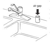
that the drain hose either be looped up and securely fastened to the underside of the counter, or be connected to an air gap.
