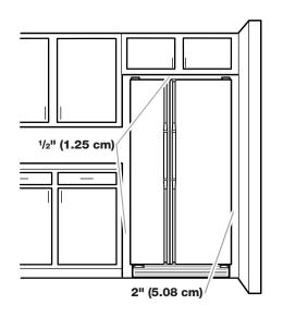
To ensure proper ventilation for your refrigerator, allow for  $\frac{1}{2}$ " (1.25 cm) of space on each side and at the top. Allow for 1" (2.54 cm) of space behind the refrigerator. If your refrigerator has an ice maker, allow extra space at the back for the water line connections. When installing your refrigerator next to a fixed wall, leave a 2" (5.08 cm) minimum space on each side (depending on your model) to allow the doors to swing open.
