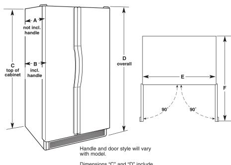
Dimensions "C" and "D" include rollers extended  $\frac{3}{4}$ " (1.9 cm).
