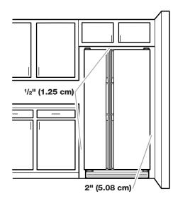
To ensure proper ventilation for your refrigerator, allow for  $\frac{1}{2}$ " (1.25 cm) of space on each side and at the top. Allow for 2" (5.08 cm) of space behind the refrigerator. If your refrigerator has an ice maker, allow extra space at the back for the water line connections. When installing your refrigerator next to a fixed wall, leave a 2" (5.08 cm) minimum space on each side (depending on your model) to allow the doors to swing open.
