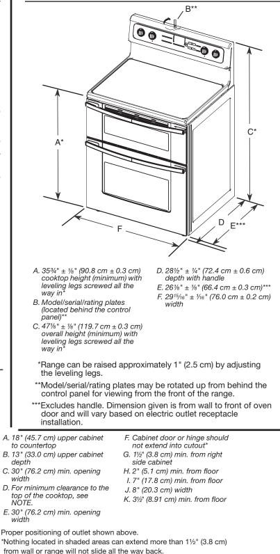
**NOTE:** 24" (61.0 cm) minimum when bottom of wood or metal cabinet is covered by not less than  $\frac{1}{4}$ " (0.64 cm) flame retardant millboard covered with not less than No. 28 MSG sheet steel, 0.015" (0.4 mm) stainless steel, 0.024" (0.6 mm) aluminum or 0.020" (0.5 mm) copper.
