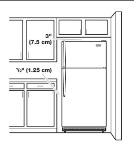
To ensure proper ventilation for your refrigerator, allow for a  $\frac{1}{2}$ " (1.25 cm) space on each side. Allow 3" (7.5 cm) of space between overhead cabinets and refrigerator top. Allow at least 1" (2.5 cm) between back of cabinet and the wall. If your refrigerator has an ice maker, make sure you leave some extra space at the back for the water line connections.
