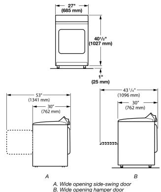
\*Most installations require a minimum 6" (152 mm) clearance behind the dryer for the exhaust vent with elbow. See "Venting Requirements."
