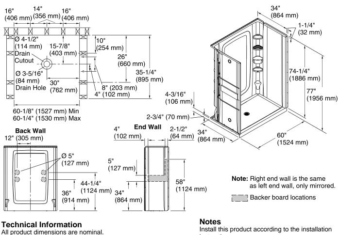
Drain hole diameter: 3-5/16" (84 mm) 29-3/16" x 56-3/4" (742 mm x 1441 mm) Basin area, bottom: 29-3/16" x 56-3/4" (742 mm x 1441 mm) Basin area, top: Minimum flat for door: 2-1/2" (64 mm) Door height required: 72-1/2" (1842 mm) Door width required: 56-3/4" (1441 mm)
