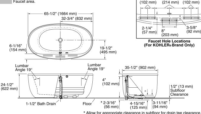
\* Allow for appropriate clearance in subfloor for drain tee clearance. Note: Horizontal PVC pipe and tee shown, not included.
