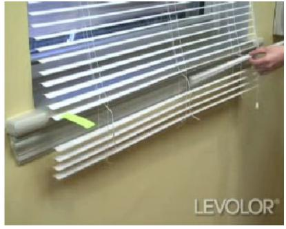
Step 6: Insert the bottom rail between the ladder cords just below the new bottom slat
