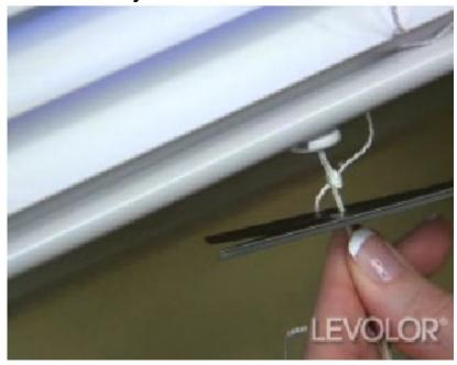
Step 8: Twist together the ladder cords and slide them into the hole in the bottom rail
