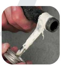
Install the gas pipe using pipe joint compound (or Teflon® tape) approved for fuel gas on all threaded connections. Keep the pipe joint compound from getting inside the gas line or gas control valve. If you are using a flexible gas line connector, follow the instructions that came with the flexible connector compound). Reconnect the gas line union.
