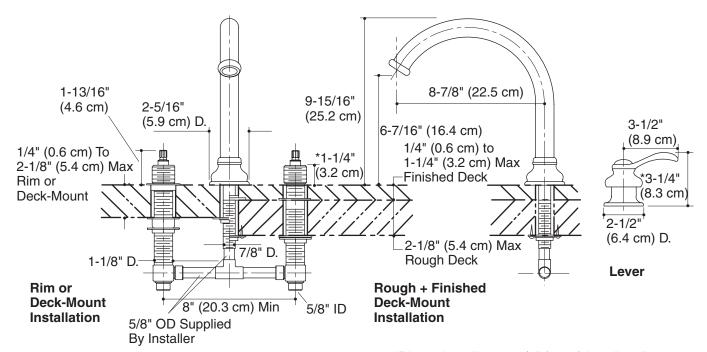
\*Dimension allows  $\pm$  1/4" (6mm) handle adjustment during handle trim installation.
