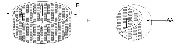
Step 3: Attach the Legs (G) to the Fire Bowl (F) using eight M6 x 12mm bolts (AA). Do not fully tighten the bolts. Insert the Decorative Rings (D) into the Leg (G) upper part, fasten them using M6 x 16mm bolts (BB). Tighten bolts once they are aligned in all the holes.
