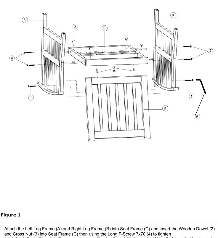
Attch Back Fram (D) to Leg Frames and insert Wooden Dowel (2) then using Short F- Screw 7x60 (1) to tighten. Tighten all F-Screw with allen wrench (5).
