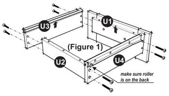
Using a <u>philips screwdriver</u>, insert 1" screws into the pre-drilled holes as shown, tighten half way. (See the figure 1)
