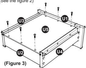
Insert the remaining (6) 1/2" screws into the pre-drilled holes on Base Part (U5), then tighten all screws.
