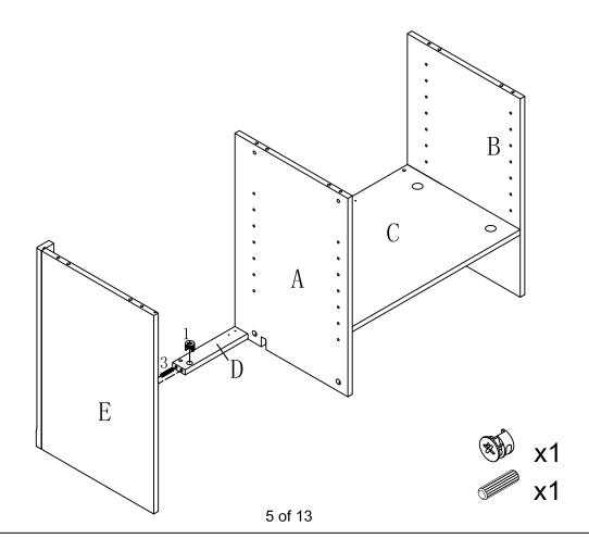
Step 5. Attach Rail G to the unit using Cam lock & Wood dowel as shown.
