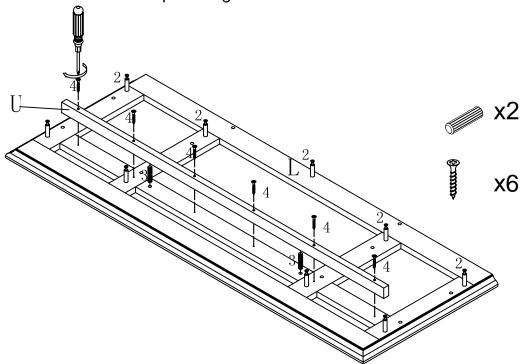
Step 10. Attach Top L to cabinet using Wood Dowels & Cam Locks as shown. Secure Rail D to Top L using one Wood Screw (Part #4) through pre-drilled hole as shown
