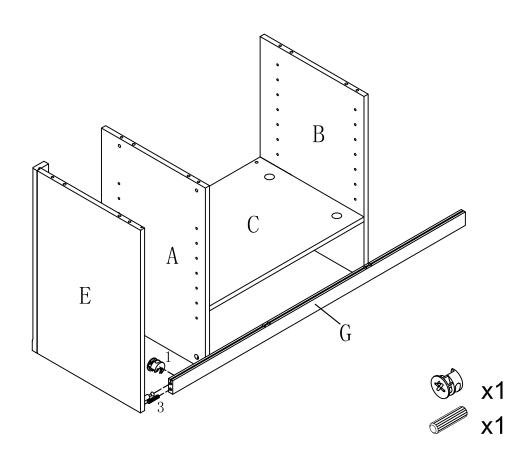
Step 6. Place Rails J into place on Rail G using Wood dowels as shown. Slide Back panels H & Panel I into the grooves as shown. Insert Wood dowels into the top end of Parts J. Attach rail G to Panel E & Rails J using Wood dowels & Cam lock as shown.
