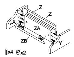
Step 10. Secure Panels J & K to Rails F & G using Screws (Part #5) & Phillips Head screw driver as shown. Attach Spice Rack (Assembled Parts X, Y, Z, & ZB) to Side Panel B using Hex Socket Head Bolts & Wood Dowels as shown. Attach Parts ZC (Towel Bar Sides) to Side Panel C using Hex Socket Head Bolts & Wood Dowels as shown. Insert Towel Bar (Part ZD) through the holes of Parts ZC. Note: Hex Socket Head Bolts will be inserted from the inside of the cabinet.
