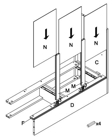
Step 5. Attach Rail H to Rails M & Side Panel C using Wood Dowels & Cam Lock as shown.
