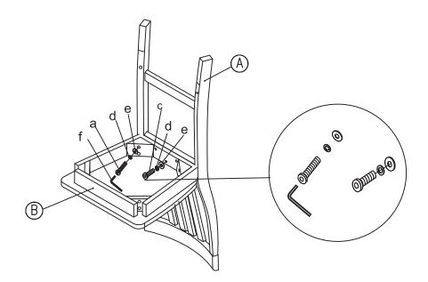
Attach left and right front legs (C) to the seat frame (B) using the bolts (b), spring washers (d) and flat washers (e) as shown in Figure 2. **Do not tighten bolts at this time.**
