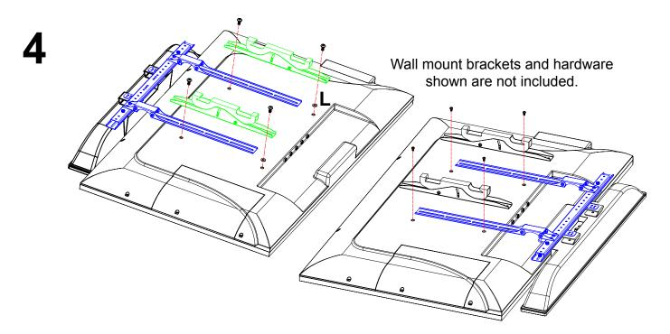
If you are installing the soundbar bracket and a TV wall mount, attach both brackets to the back of the TV using TV mount screws. If vertical bars (A) do not extend over the bottom two TV mounting holes, use spacers (L). The soundbar can be mounted above or below the TV as shown.
