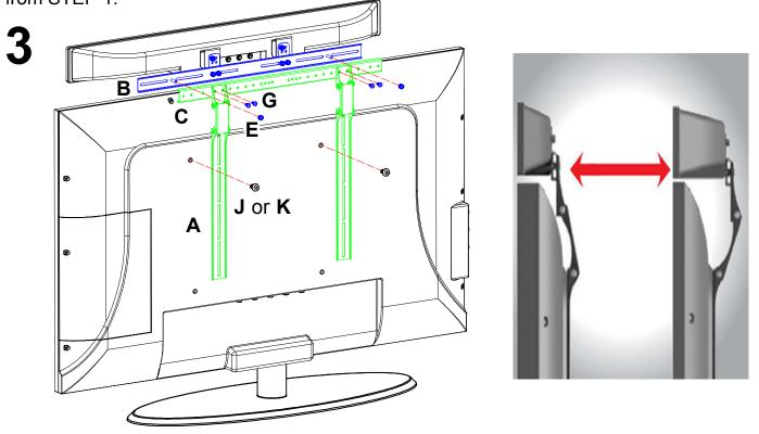
Attach vertical bars (A) to horizontal bar (C) with screws (G). Attach bars (A) to TV back with screws (J or K). Join horizontal bars (B and C) with nuts (E). Adjust soundbar position as shown above.
