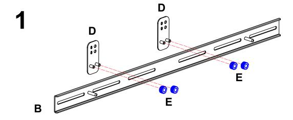
Check the soundbar hole spacing. Then attach the sliding plates (D) onto the horizontal bar (B) with nuts (E), but do not tighten them.
