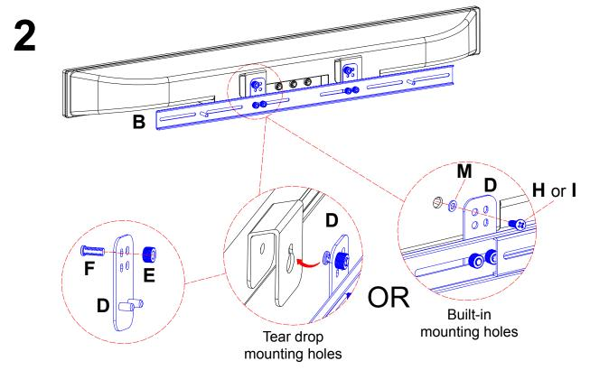
For a soundbar with tear drop mounting holes, attach sliding plates (D) to the soundbar with screws (F) and nuts (E). For a soundbar with built-in mounting holes, attach the sliding plates (D) to the soundbar with screws (H or I) and washers (M). Tighten the four nuts (E) from STEP 1.
