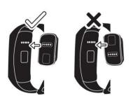
Insert the micro-USB cable into the charging cradle, and then connect the USB plug into a power source. A "Charging" icon will be shown on the screen and will indicate the current charge level.
