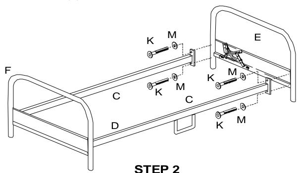
CAREFULLY ATTACH REAR CROSS RAIL (C) TO BACK POST OF THE RIGHT SIDE PANEL (E), SECURE IN PLACE USING 2 SHORT ALLEN BOLTS (K) AND 2 METAL WASHERS (M). NEXT ATTACH FRONT CROSS RAIL WITH CENTER SUPPORT (D) TO FRONT POST OF THE RIGHT SIDE PANEL (E), SECURE IN PLACE USING 2 SHORT ALLEN BOLTS (K) AND 2 METAL WASHERS (M).
