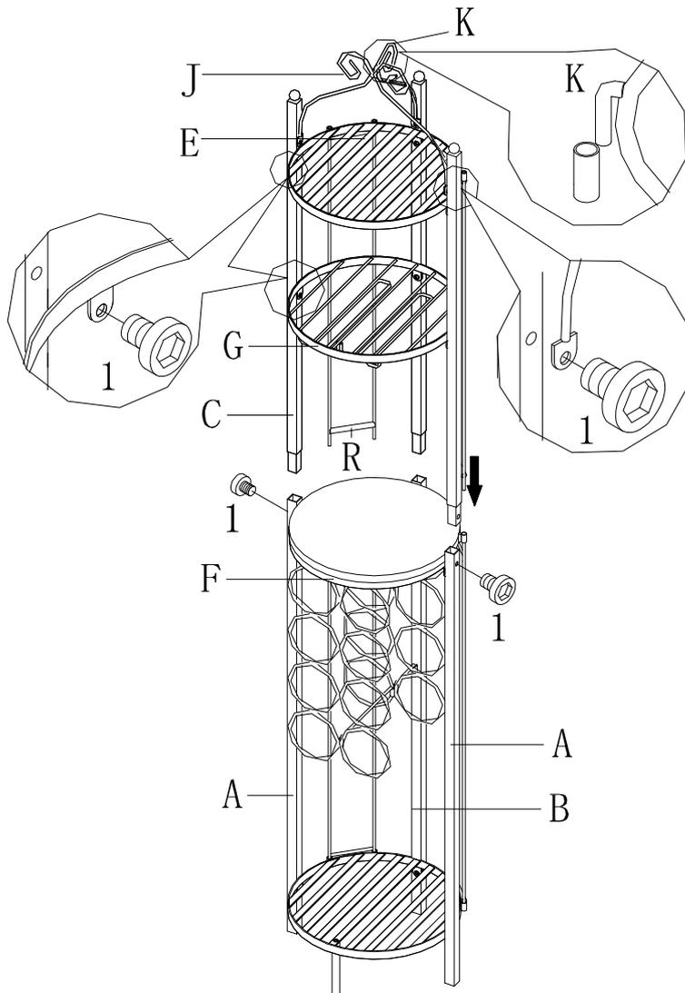
Put 3pcs Upper tube(C) into bottom tube(A & B),then inster 3pcs bolt(1) through holes on bottom tube(A & B) to attach upper tube( C) to bottom tube(A & B).
