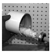
Apply a second full coat of cement to the pipe surface aggressively working it in.
