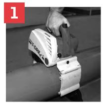
chanical cut off saw with carbide tipped blade or other appropriate tool.
