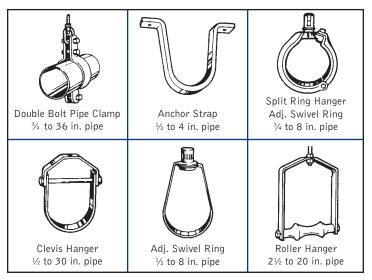
The pipe should not be anchored tightly by the support, but secured in a manner to allow for movement caused by thermal expansion and contraction. It is recommended that you use clamps or straps that allow pipe to remain away from the framing, thus reducing the noise generated when pipe is allowed to rub against wood.
