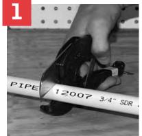
Acceptable tools include ratchet type pipe cutter,
