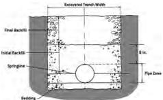
Additional information is contained in ASTM D 2321 "Underground Installation of Thermoplastic pipe for Sewers and Other Gravity-Flow Applications" (non-pressure applications) and in ASTM F 1668 "Construction Procedures for Buried Plastic Pipe." ASTM Standards are copyrighted documents and can be purchased from ASTM International: 100 Barr Harbor Drive West Conshohocken, PA 19428 or "http://www.astm.org."
