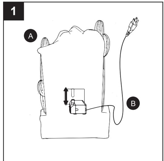
2. Ensure the power cord of pump (B) is out of the item, then fill base (A) with clean water. Note: The maximum water level should be approximately 1.2 inches below the top edge of base (A).
