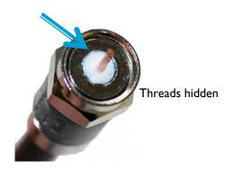
4) Cable is fully seated when white dielectric is flush with the bottom of the nut.
