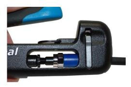
5) Place NJX connector in standard F compression tool and compress. The post slides backwards. This connector does not get shorter in length.
