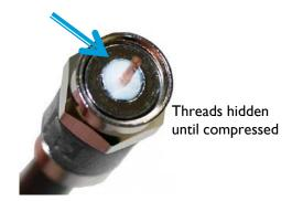
4) Cable is fully seated when white dielectric is flush with the bottom of the nut.
