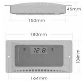
Depth 45mm (1.77in) width 180mm (7 in) length 104mm (4.1 in) Distance between holes for mounting 164mm (6.5 in) Net weight is approximately 350g
