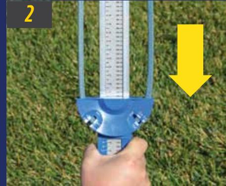
Place the other end of the belt in the bottom guide and stretch the belt as much as you can by pulling downward.
