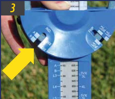
Determine the belt width using the markings on the side of the lower guide. (This example is an "A" Belt)
