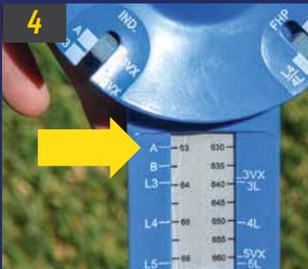
Determine the length by first locating the markings that correspond with the width, then on the left side, in-line with that marking, you'll see the fractional belt number.
