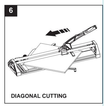
6. Position the tile at 45°, then, using proper pressure, score the tile one time from rear corner to front corner.
