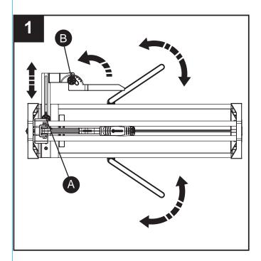
Position the extension arms, side rule (release knob A) and angle guide (release knob B) as desired to support stable positioning of tile (not included) for scoring.
