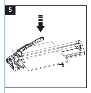
Align the breaker bar with tile front edge, then press the grip handle.
