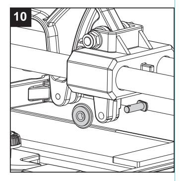
10. Remove the dulled cutting wheel.
