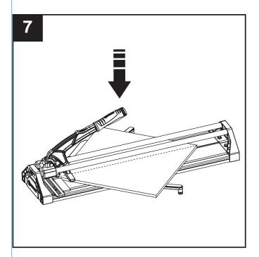
7. Align the breaker bar with tile corner, then press the grip handle.
