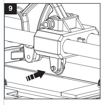
Push out the collar pin. The collar pin may require a strong push to be removed.
