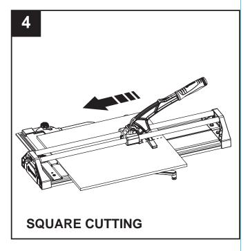
4. Mark the tile to be cut at proper width. Position the tile at 90°, then, using proper pressure, score the tile one time from rear edge to front edge.
