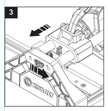
There is a lock on the front support (unlock it to release the grip handle before start using) which will hook the grip handle during movement of the tile cutter to avoid any sliding and impact.
