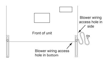
WIRING/CONDUIT CONNECTIONS FOR REMOTE/IN-LINE BLOWER
