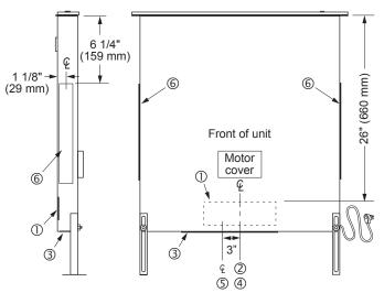
2" X 16", connects to side or bottom exhaust on raised vent
