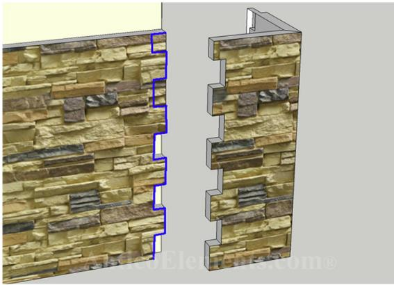
Now place the corner over the last panel and, with a marker, trace the "fingers" of the corner over the panel. Using a jig saw create the fingers on the panel to match those of the corner. Some filing and sanding will be necessary to create a snug fit. Try to cut on or inside the marked lines to avoid gaps. In some cases it may be necessary to remove the flat "lip" on the panel or corner that is not getting cut, to create a flat and even seam.
