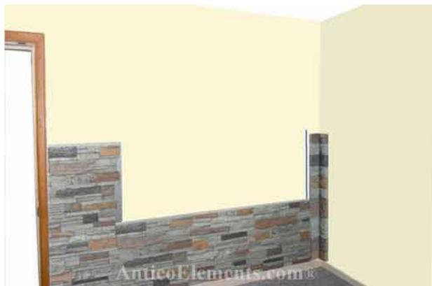
If installing multiple rows of panels, we strongly advice to cut the first panel of the next row in half, and use the half with the straight lip. This is needed to stagger the vertical seams. ( This doesn't apply for Castello and Corallo Panels )
