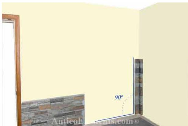
We recommend that you install the panels from left to right (for the Laguna panels it would be right to left). For better results mark some horizontal chalk lines on the wall to keep your panels leveled.
