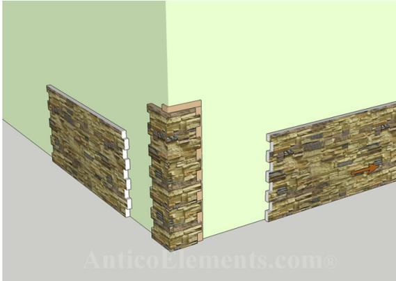
Temporarily place the first corner with one screw ( you might need to remove it later if you install a panel on the left side ). The above image shows the 36" high Interlocking Corner but we also have the 24". The top of the corner has the 3/4" high lip, the bottom has a notch in the back
