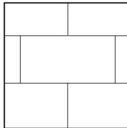
Stagger butt end (cut end) joints so joint does not extend across the ceiling. Never place a butt end next to a tapered edge.
