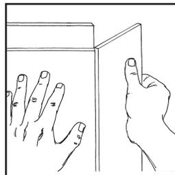
Snap board along the score over the edge of a solid support. (A quick action produces the best results.)
