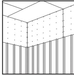
Hold the lower sidewall panel snugly against upper panel. A panel lifter (as shown) will help hold the panel until fastened. Begin fastening near the center of board and proceed to the outside.
