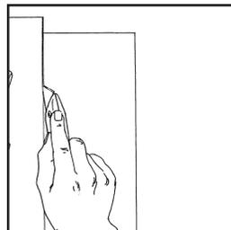
Using a straightedge and utility knife, score the drywall on the face paper side along the pencil line(s).
