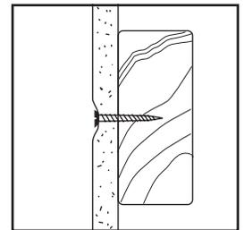
Slightly recess the nail or screw head. Indent face paper without tearing it.
