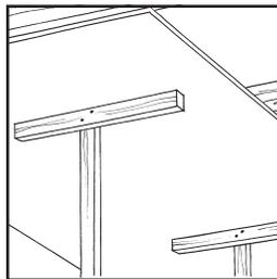
Start with ceiling, applying drywall at right angles to joists. Use panel lifter or a temporary T-brace to support weight.
