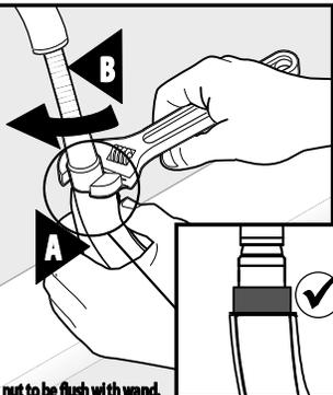
Tighten hose nut to be flush with wand.
